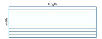
L – longitudinal, when parallel with the glass sheet lenght.
