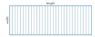
T – transversal, when perpendicular with the glass sheet length.
